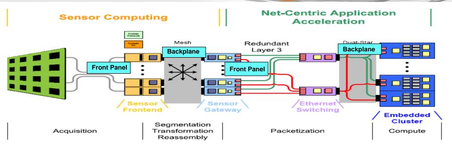
RADAR, sonar, video, etc. sensors Sensor compute modules (FPGA) A to D converters, RF tuners VITA 41, 46/48, OpenVPX – 3U, 6U, SBC modules DSP modules (PPC / x86 multicore, GPU) Switch module (e.g., serial RapidIO – sRIO)
