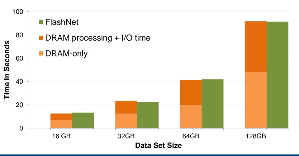
FlashNet adds minimum overheads to RDMA-ready applications
