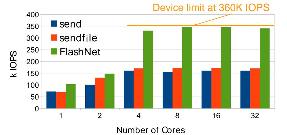
FlashNet IO operations scale better wrt per-core scaling
