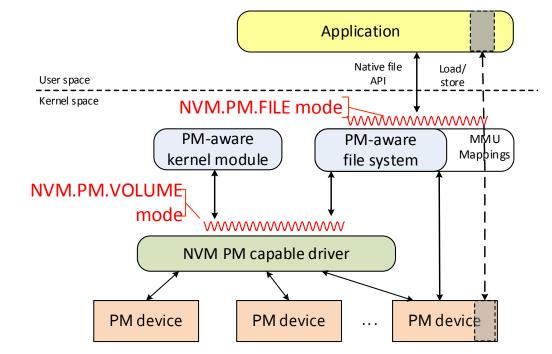
Memory Mapping in NVM.PM.FILE mode enables direct access to persistent memory using CPU instructions
