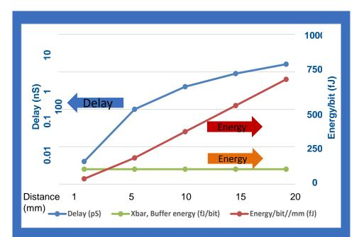
Cross die wires will need to be buffered Logic (switches) at clock cycle intervals Local BW is cheap, cross die BW will cost time and energy; optimize for locality
