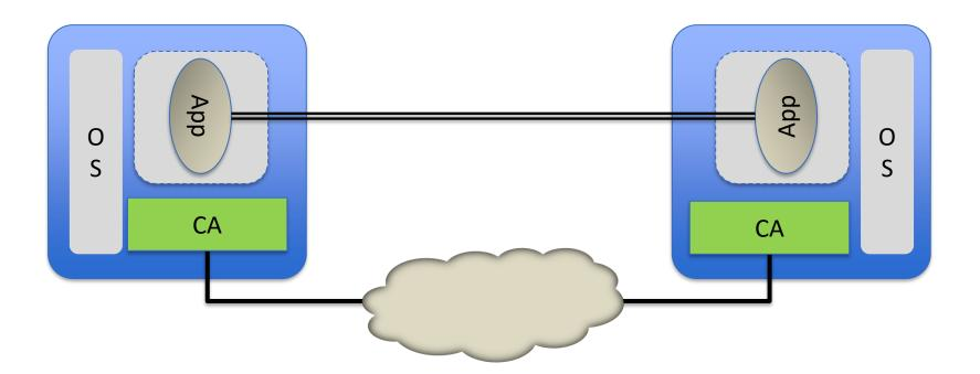
A channel spans disjoint physical address spaces That's why the RDMA messaging service is built on a networking model Networks allow communication between disjoint physical address spaces
