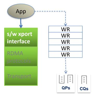
A <u>Work Request</u> (WR) is a data structure that describes a piece of work to be completed: -a message to be sent, -a message to be received...
