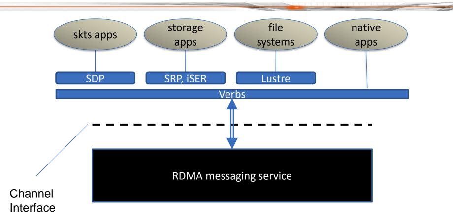
The channel interface provides a consistent programmatic interface to the message passing service
