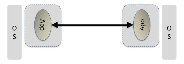
An I/O Channel connects virtual address spaces. The virtual address spaces can exist in disjoint physical address spaces.
