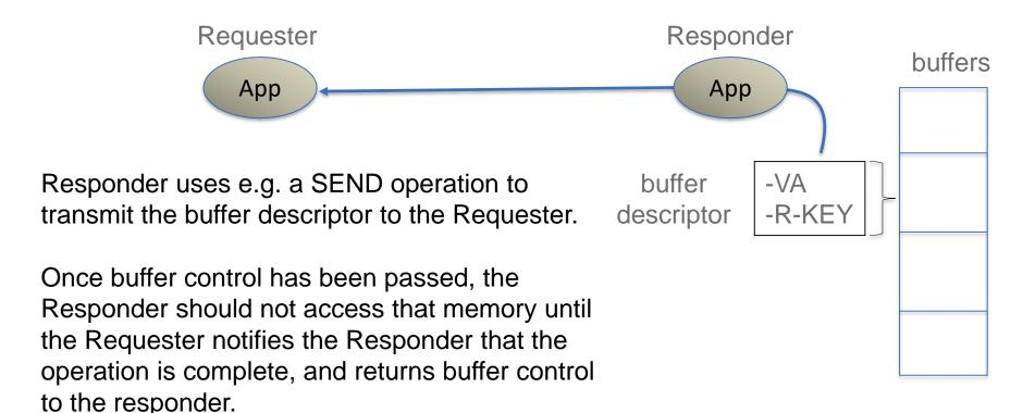
The means for passing control of the buffer back and forth is not specified in the RDMA architecture; it is defined by the upper layer protocol
