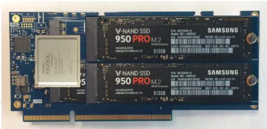
CF-NVMe-v2 (FPGA + 2x2TB) (256TB per chassis / 4 PB per rack)
